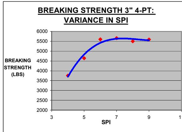
**Graph 3:** Effect of SPI on Breaking Strength
