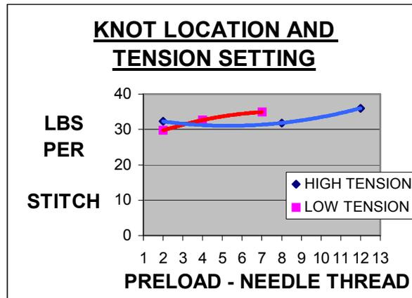
**Graph 7:** Effect of knot location and tension setting
