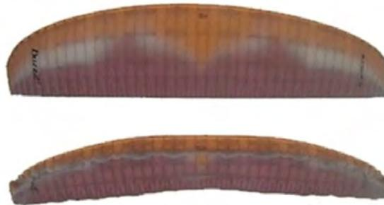
**Fig. 31.20** Demonstration of a B-Line Stall in a Paraglider
