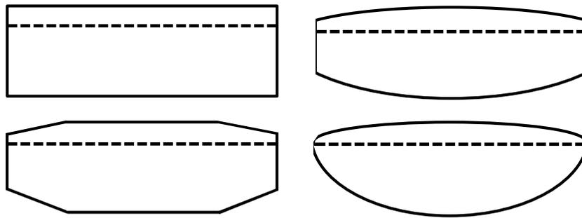
**Fig. 31.5** Planform Shapes: Rectangular, Polygonal, Semi-elliptical and Fully Elliptical.
