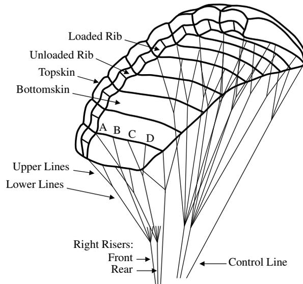
**Fig. 31.1** Ram-Air Wing Components
