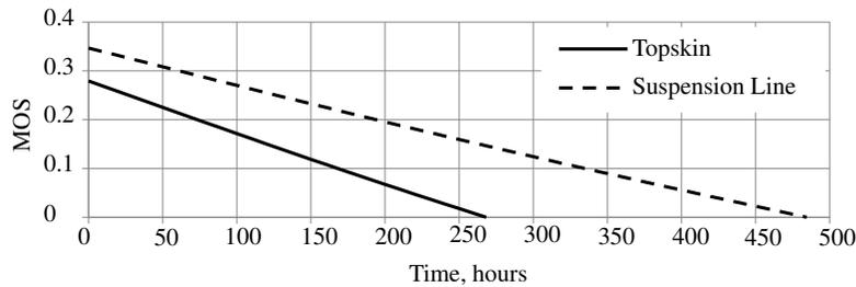
**Fig. 31.23** Example Ram-Air Wing Margins of Safety (MOS).
