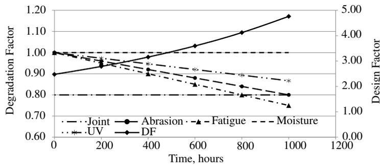
**Fig. 31.22** Example of Suspension Line Degradation Factors and Resultant Design Factor (DF).
