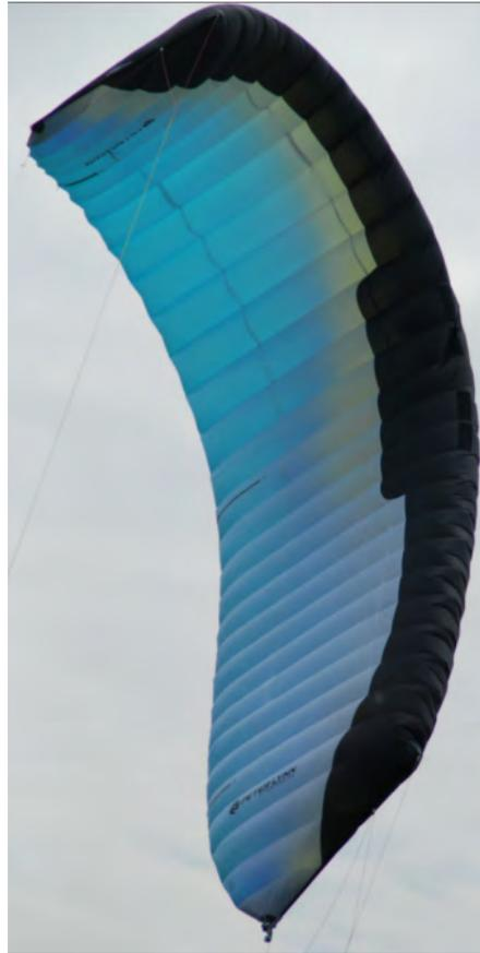
**Fig. 31.17** Flagging of a Four-line Ram-Air wing, Mid-process (Photo by Delft University of Technology).
