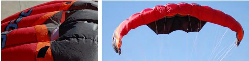
**Fig. 31.16** Topskin and Bottomskin Spoilers Used to Explore Glide Modulation.
