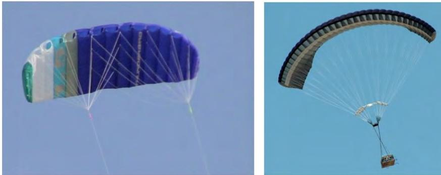
**Fig. 31.14** Images of Steering via Left Right Asymmetry and Steering via Control Lines (Left Photo by Storm Dunker, Right Photo by Steve Tavan, US Army).
