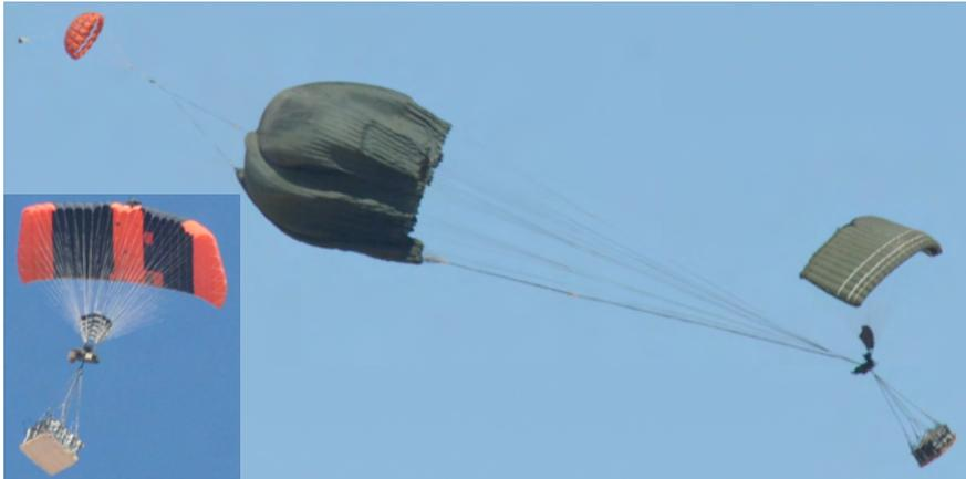
**Fig. 31.11** Highly Loaded Screamer Ram-Air Wing (Photos by Steve Tavan, US Army).
