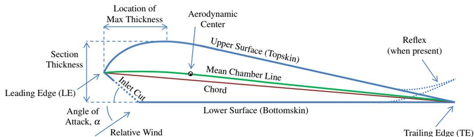
**Fig. 31.3** Basic Parachute Ram-air Airfoil Diagram; Paraglider LE's are typically more rounded with a shallower inlet cut, made possible using stiffeners such as Mylar or flexible rods. Often, the lower surface has curvature upward near the inlet cut.
